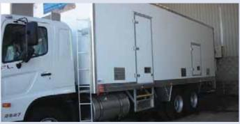
Our external trim consists of a variety of heavy-duty aluminium angles and channel to doorways. We use a heavy duty base rail, giving maximum support to the walls of the body in critical areas. Polished and anodised are available. Alloy mudguards are fitted to each body as a standard feature.
