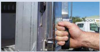
Rear and side doors are made with alloy trim, stainless steel hardware, camlocks and offset hinges to allow the doors to fully open and latch to body sides. Rear door frames are manufactured from either stainless steel or hot-dipped galvanised steel, depending on structural requirements. This provides extra reinforcement for heavy-duty work.
